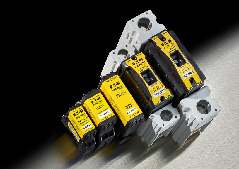
The Bussmann series CUBEFuse holder is a finger-safe\* modular system of single-pole 30, 60, 100, 200, 225 and 400 amp holders. All holders can be dovetailed together to create the desired number of poles for the application, with 30, 60 and 100 A holders able to have mixed amp ratings.
