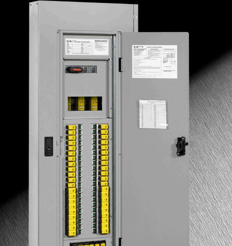
The Bussmann series QSCP provides up to 200 kA SCCR while requiring 40% less space than traditional fusible panelboards. Highly configurable, the QSCP is available in NEMA 1 and 3R enclosures, and can be used as a branch circuit or UL service entrance panel in systems up to 600 Vac.
